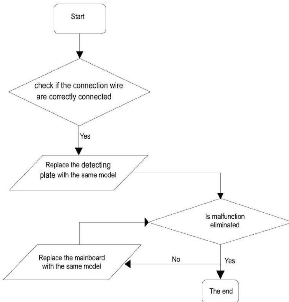
**2. IPM protection(H5), desynchronizing malfunction(H7), overcurrent of compressor phase current (P5) (AP1 below means control board of outdoor unit)**
