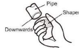
**C: Put on suitable insulating pipe**
